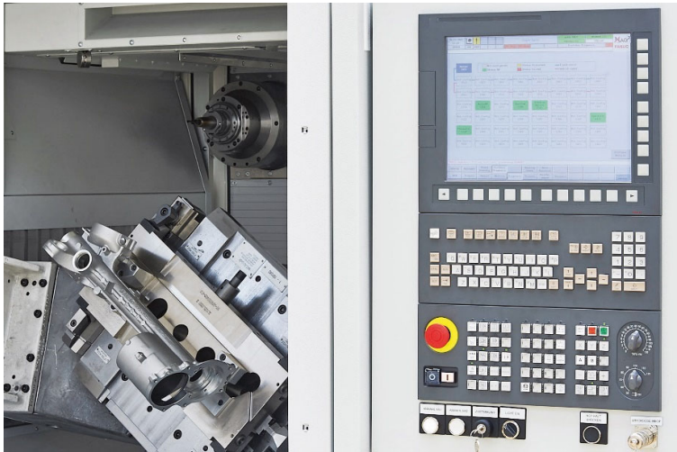
Figure 5: Complete machining of a steering housing in one setup with adapter plate and dry machining with minimum quantity lubrication (MQL). Image download: http://pr-x.de/fileadmin/download/pictures/MAG/Komplettbearbeitung_Lenkgehaeuse.jpg
