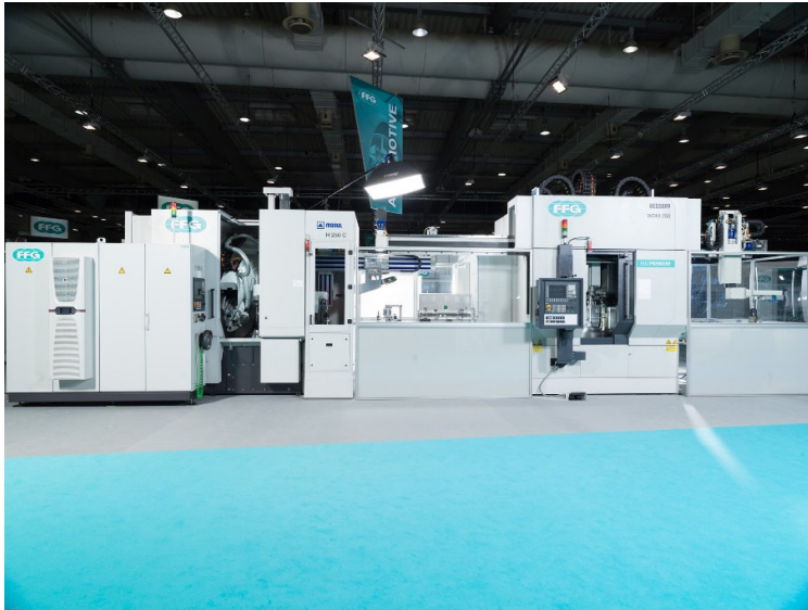
Figure 7: Production cell for soft machining of a shaft with splines consisting of a HESSAPP WDM 250 vertical lathe and a MODUL 250 C gear hobbing machine with integrated deburring station Image download: http://pr-x.de/fileadmin/download/pictures/MAG/HESSAPP_WDM_250.jpg
