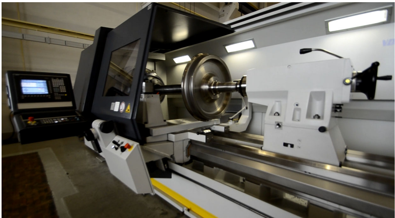
Figure. 14: Horizontal CNC lathe BOEHRINGER VDF 1110 DUS for machining wheelsets for profiling the wheels and machining the brake disc surfaces
